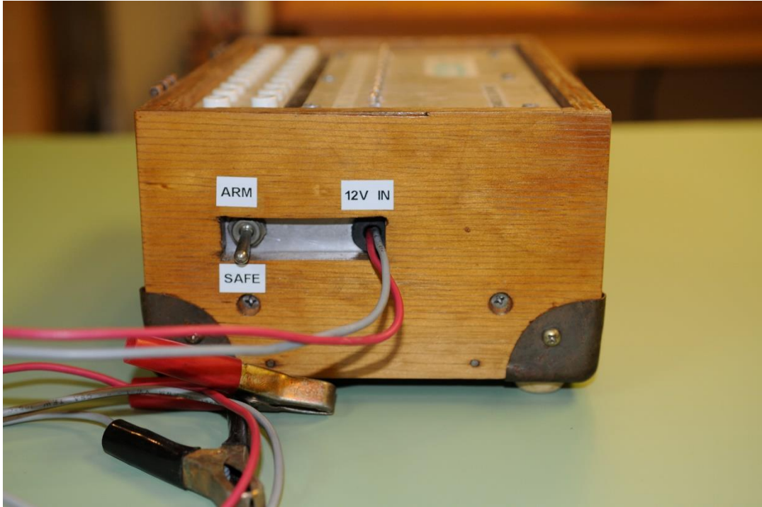
Photo 8: Firing Box ARM/SAFE Switch
