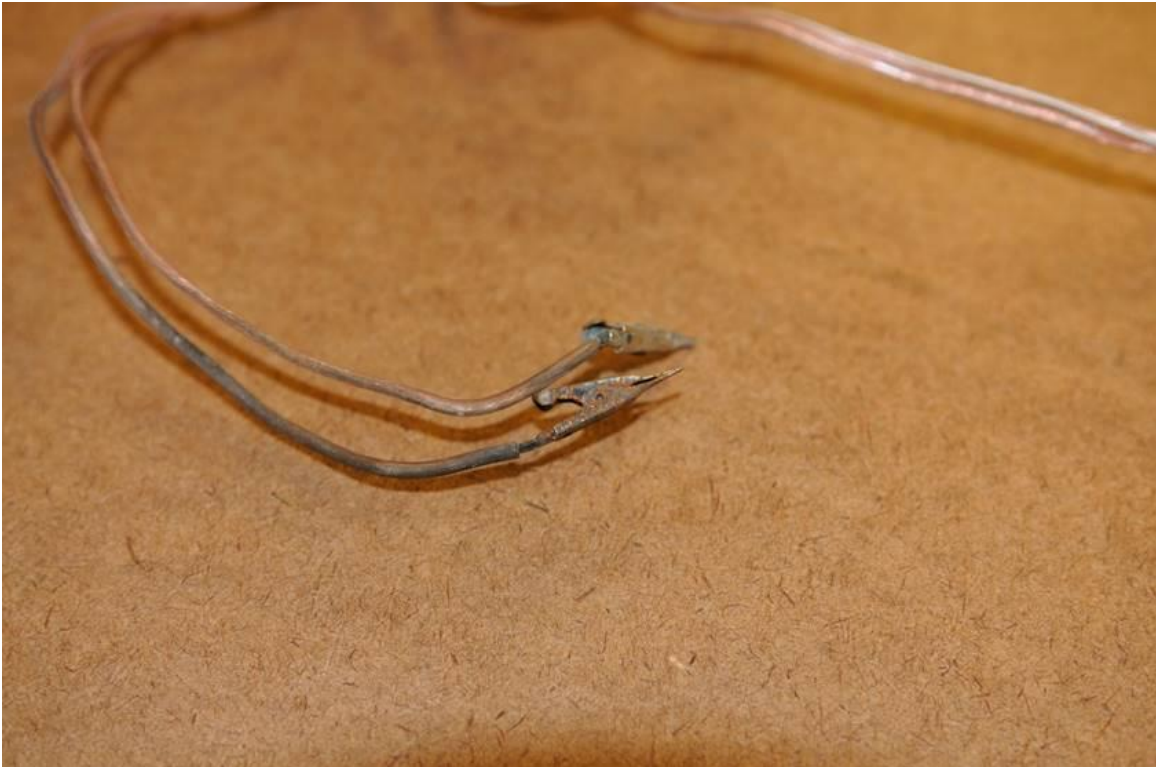
Photo 1: Corroded Igniter Lead Clips
